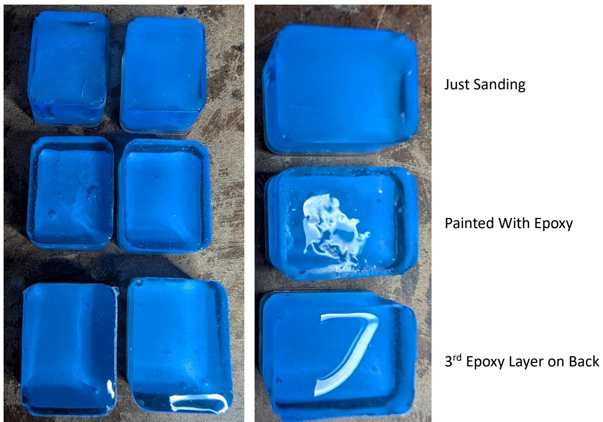
Figure 1-18. Back Finishing Approach Results (top: light sand, middle: paint with clear epoxy, bottom: add epoxy layer)
