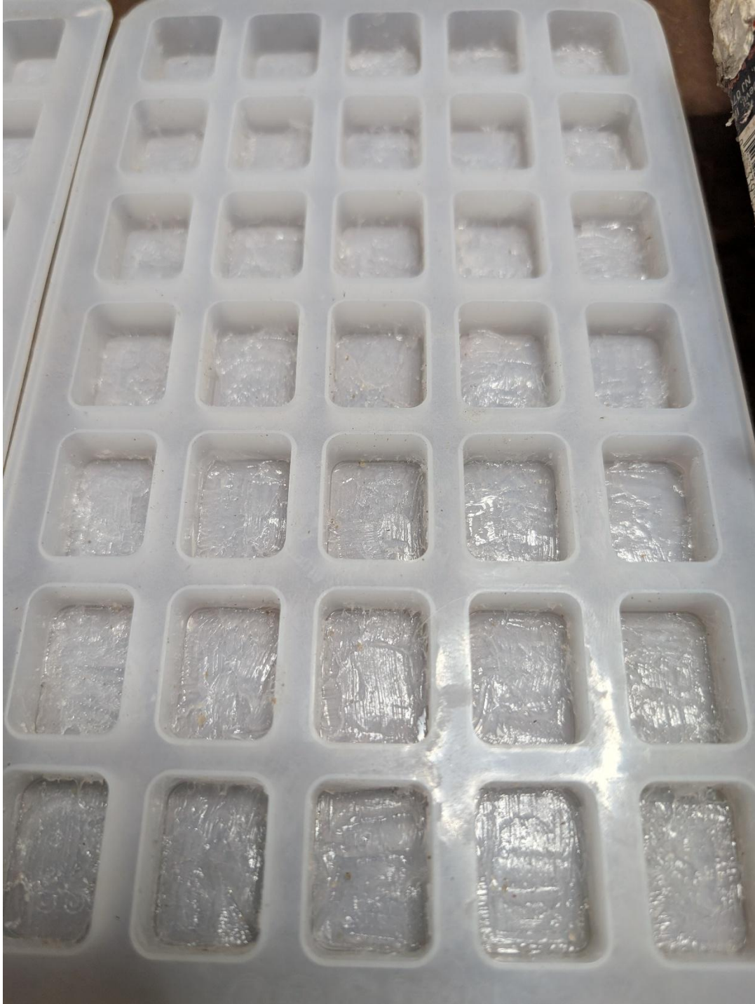
Figure 1-2. Mold with Silicone Glue Applied
