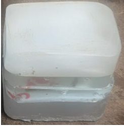
Figure A-1. Cutting and Sanding Block Made from 2 Tiles Glued Together
