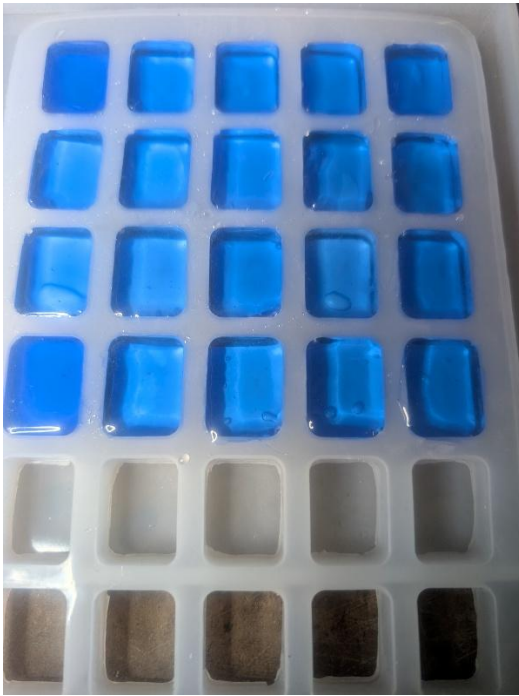
Figure 1-19. Special Mold Constructed to Add Another Bottom Layer
