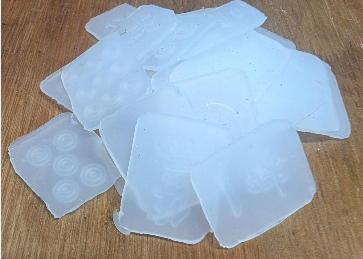
Cut Mold Pieces Can Be Used to Make a Modified Mold with Shallower Trays
