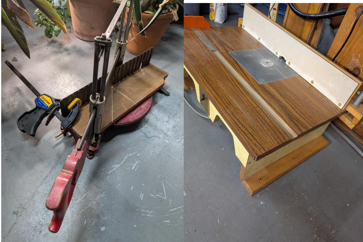
Figure 3. Miter Box with Hand Saw and Clamp (L) and Router Table (R)
