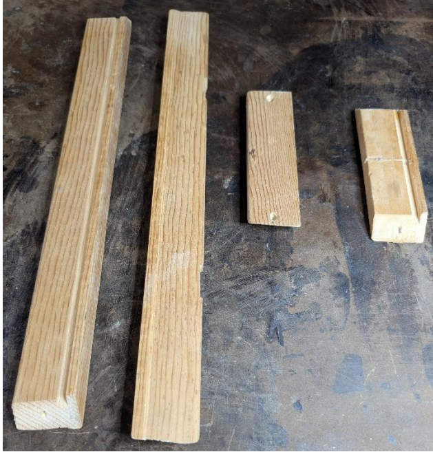
Figure 4. Cut and Routed Side Pieces
