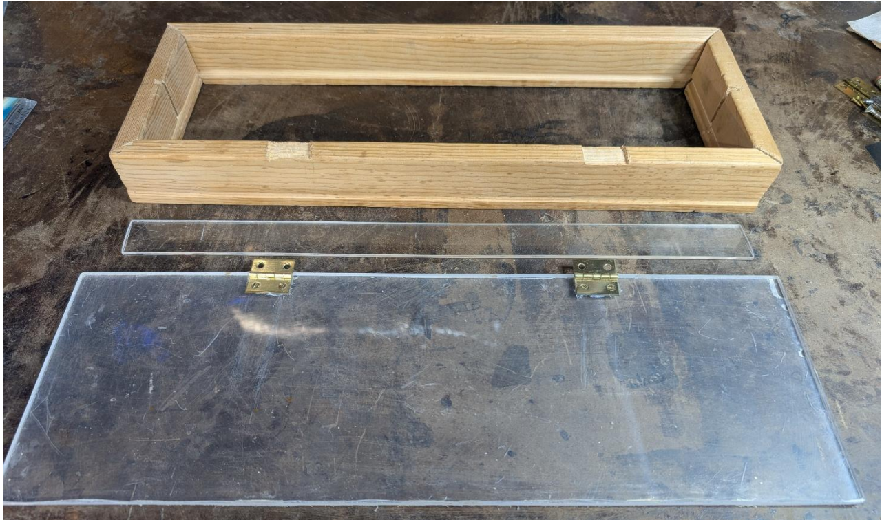
Figure 8. Top with Hinges Attached and Box with Hinge Grooves Cut
