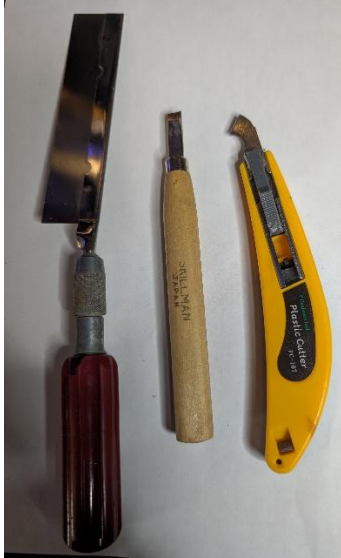
Figure 5. More Cutting Tools – Craft Saw, Wood Chisel, Plastic Cutter (L to R)
