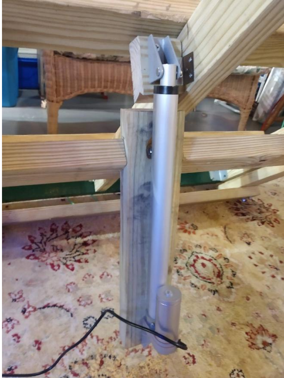
Figure 4.1-3. Mounting Boards with the Actuator Mounted.
