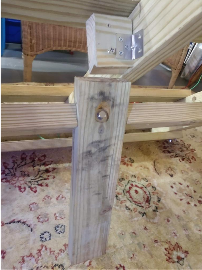
Figure 4.1-2. Mounting Boards Installed Before Mounting the Actuator.
