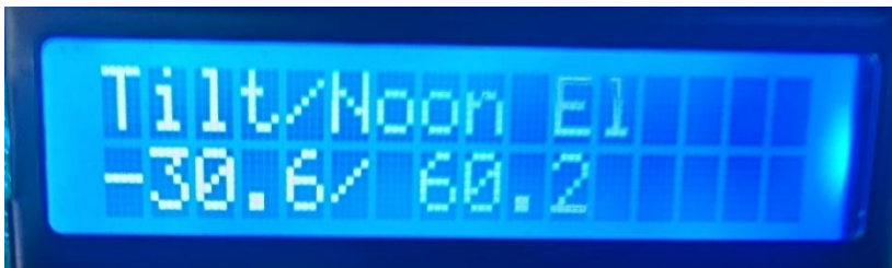
Figure 3-9. Current Tilt and Maximum Sun Elevation Display Example.
