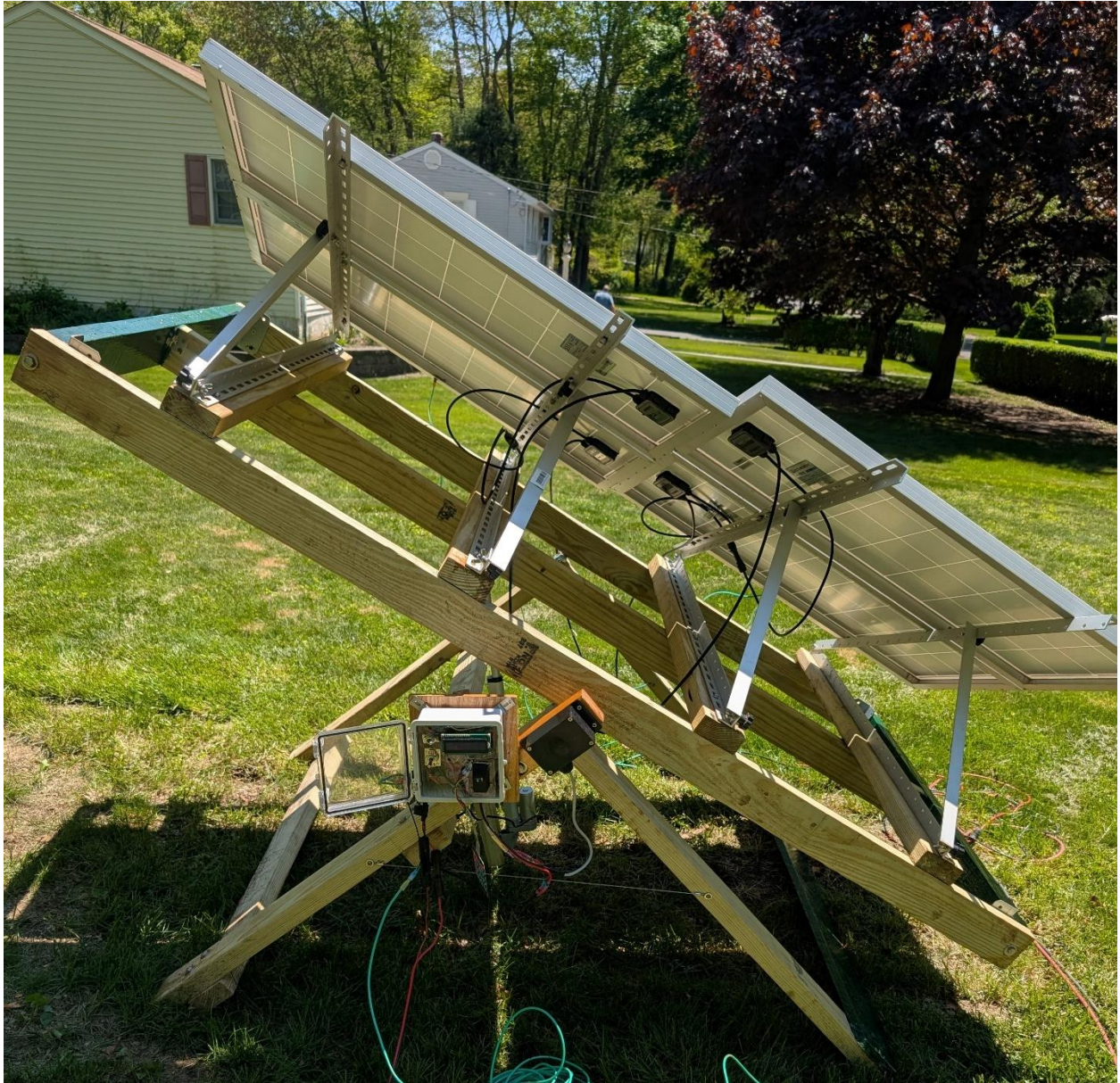
Figure 2-14. Base with Panels Mounted Outside, Back View.
