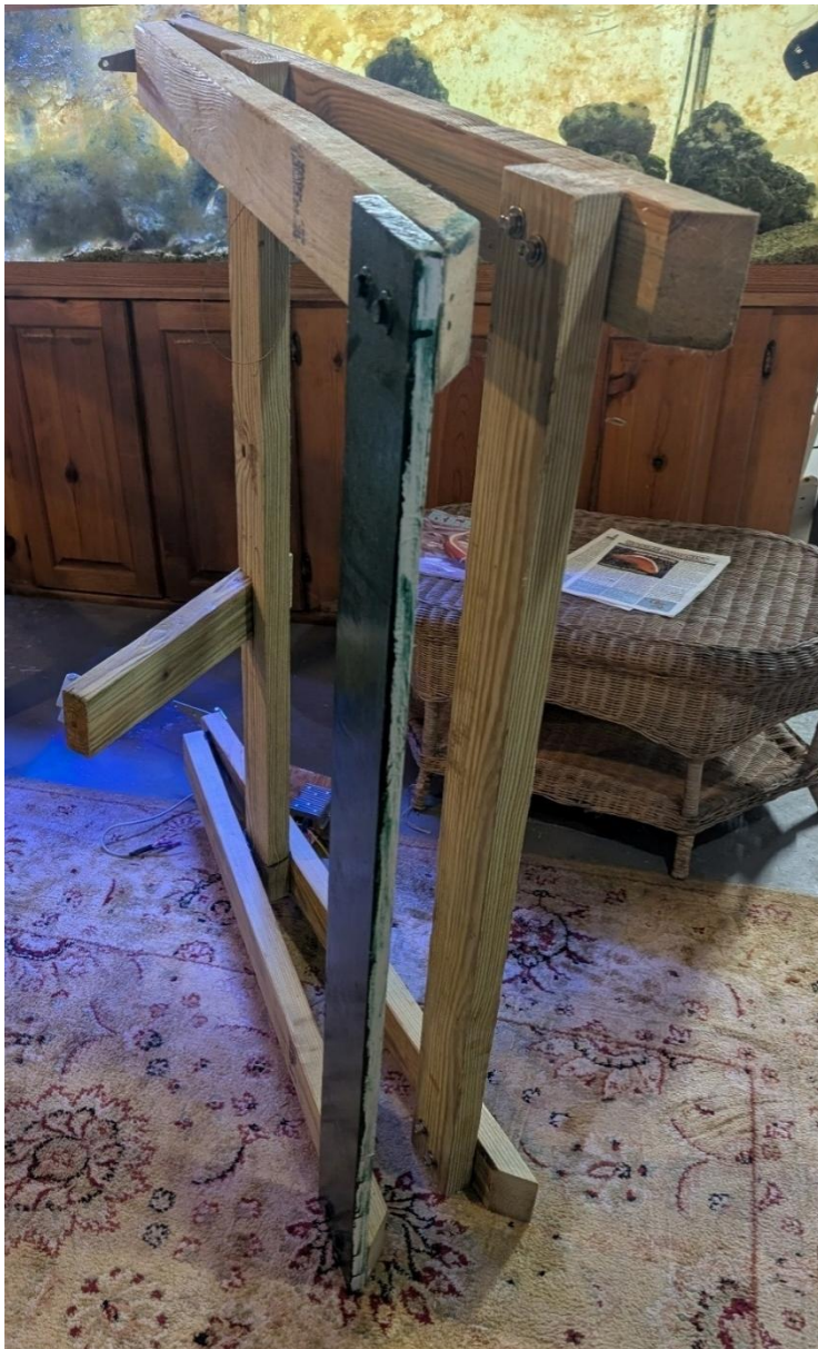
Figure 2-9. Disassembled and Folded Lower Base.
